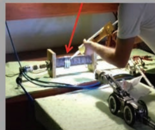
FIXATION OF DAMAGE SEAM
